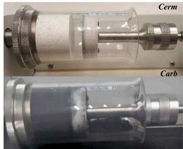
Fig. 7. Powder pycnometry analysis employing the envelopers.
